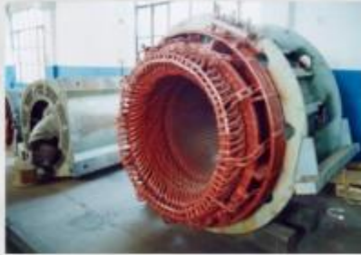
10MW,11KV MOTOR STATOR REWIND
