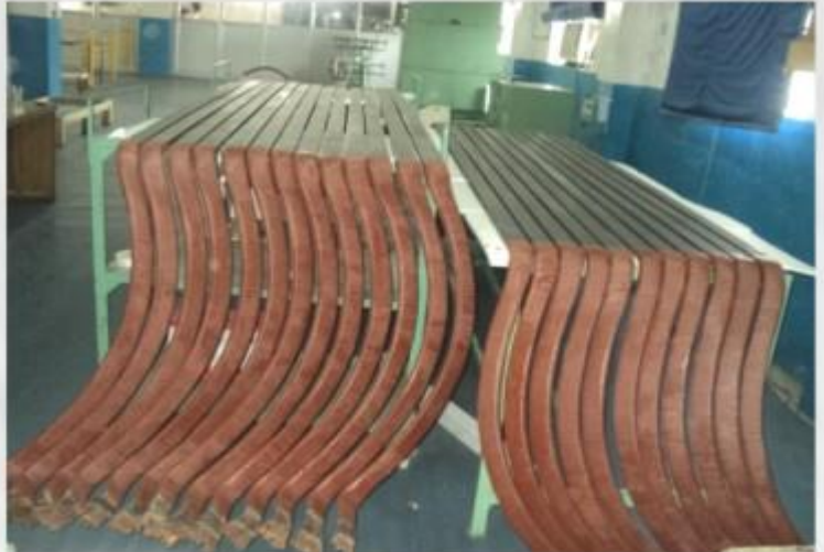
25MW,11KV,2P ROEBEL BARS FOR ON-SITE STATOR REWIND
