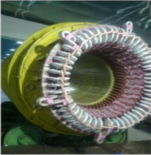
25MW,11KV STATOR AFTER REWIND
