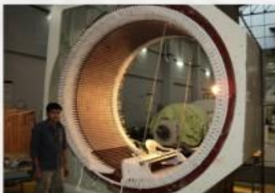
10MW,11KV HYDRO-STATOR REWIND ( AT SITE)
